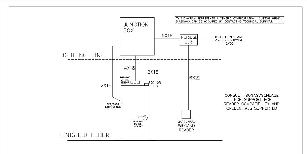
1) ALL LOW VOLTAGE WIRING TO BE STANDARD, MULTI-CONDUCTOR COLOR CODED WITHOUT SPLICES.
