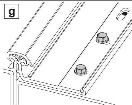
g. Tighten all screws on door leaf. Reconnect the closer and any other hardware.
