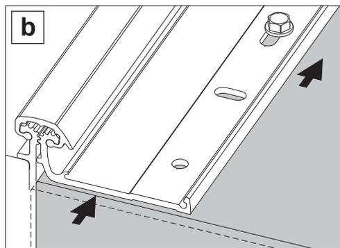
b. Use pry bar to raise door until tight against shims between the top of door and frame header.
