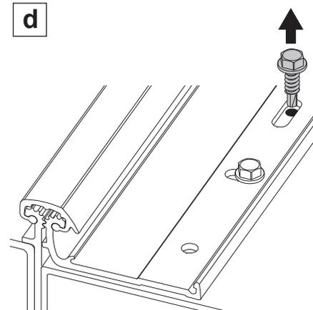
d. Remove shims from top of door(s) and remove screws from vertical slots.
