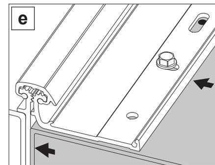
e. Adjust lateral clearances of door by prying door from lock side of frame. For double doors, make sure they remain centered.
