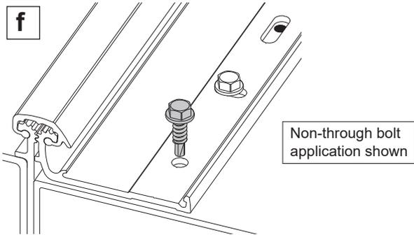
f. Install screws into two or three round holes at both top and bottom of hinge. Open and close door slowly, checking all edges for clearance. Repeat for double doors.
