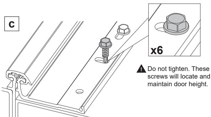
c. Install screws into lock side end of each horizontal slot. Repeat for double doors.
