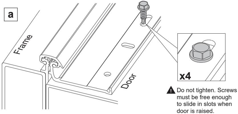
a. Fold door leaf of hinge against door. Install a hex screw at the bottom end of each vertical slot.
