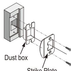
Use the strike plate as a template to drill the latch and screw holes and chisel out the mortise. The strike plate must fit flush with the surface of the door jamb. The hole must be at least 1" (25mm) deep.
