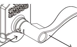
Insert pin wrench into small hole near base of lever, then pull lever to remove. Remove both levers, then reinstall levers to the opposite side they were removed.
