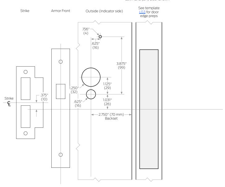
Refer to Template [G] for case and strike dimensions and if applicable information to prepare the door for wire routing. Armor front deadbolt, auxiliary latch and latchbolt holes shown for dimensional purposes only. Use door edge measurements for door preparation.
