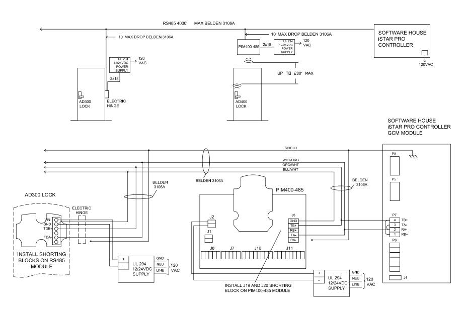
NDTES: 1) ALL LOW VOLTAGE WIRING TO BE STANDARD, MULTI-CONDUCTOR COLOR CODED WITHOUT SPLICES.
