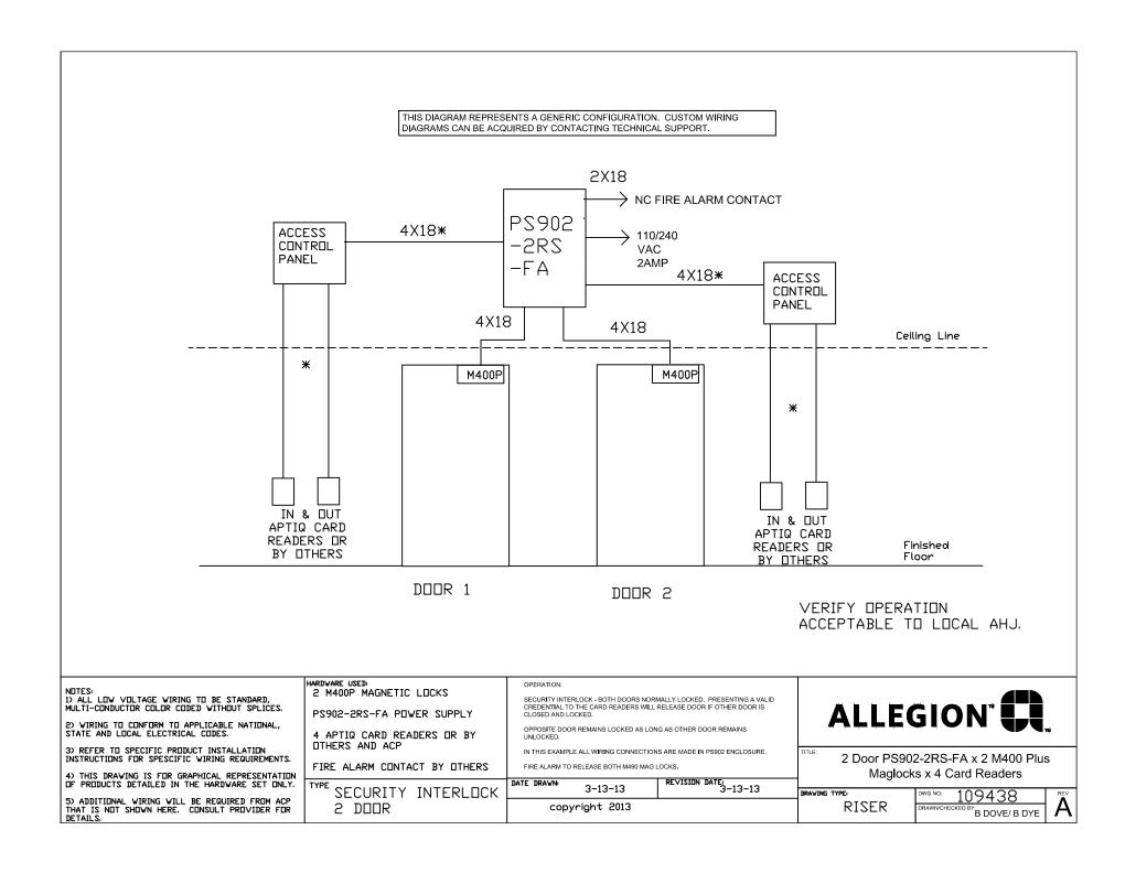
THIS DIAGRAM REPRESENTS A GENERIC CONFIGURATION. CUSTOM WIRING DIAGRAMS CAN BE ACQUIRED BY CONTACTING TECHNICAL SUPPORT.
