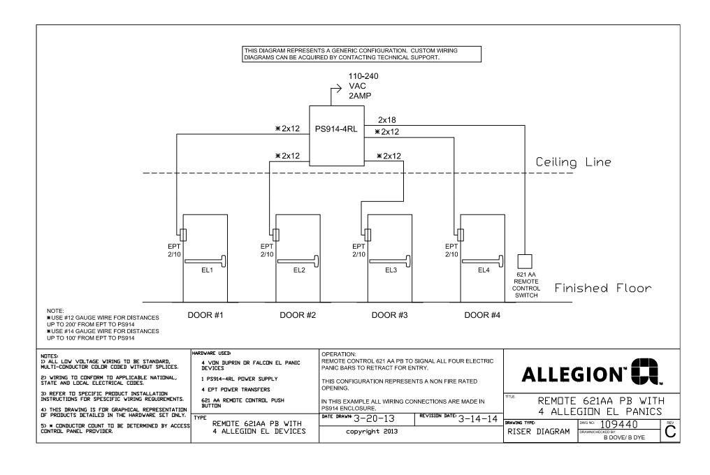
THIS DIAGRAM REPRESENTS A GENERIC CONFIGURATION. CUSTOM WIRING DIAGRAMS CAN BE ACQUIRED BY CONTACTING TECHNICAL SUPPORT.
