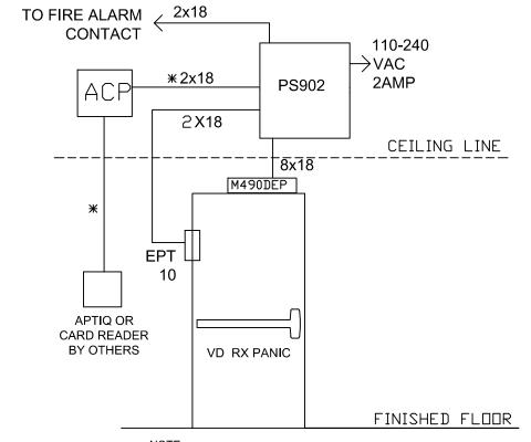
THIS DIAGRAM REPRESENTS A GENERIC CONFIGURATION. CUSTOM WIRING DIAGRAMS CAN BE ACQUIRED BY CONTACTING TECHNICAL SUPPORT.
