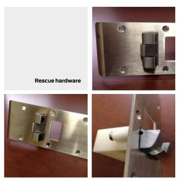
Rescue hardware used in conjunction with center hung pivots ensures a door can be accessed by allowing the door to swing the other way. Basically, it acts like a door jamb and swings in one primary direction in normal use. In an emergency situation, it depresses the center tong and allows the door to move in the opposite direction without damaging the frame.
