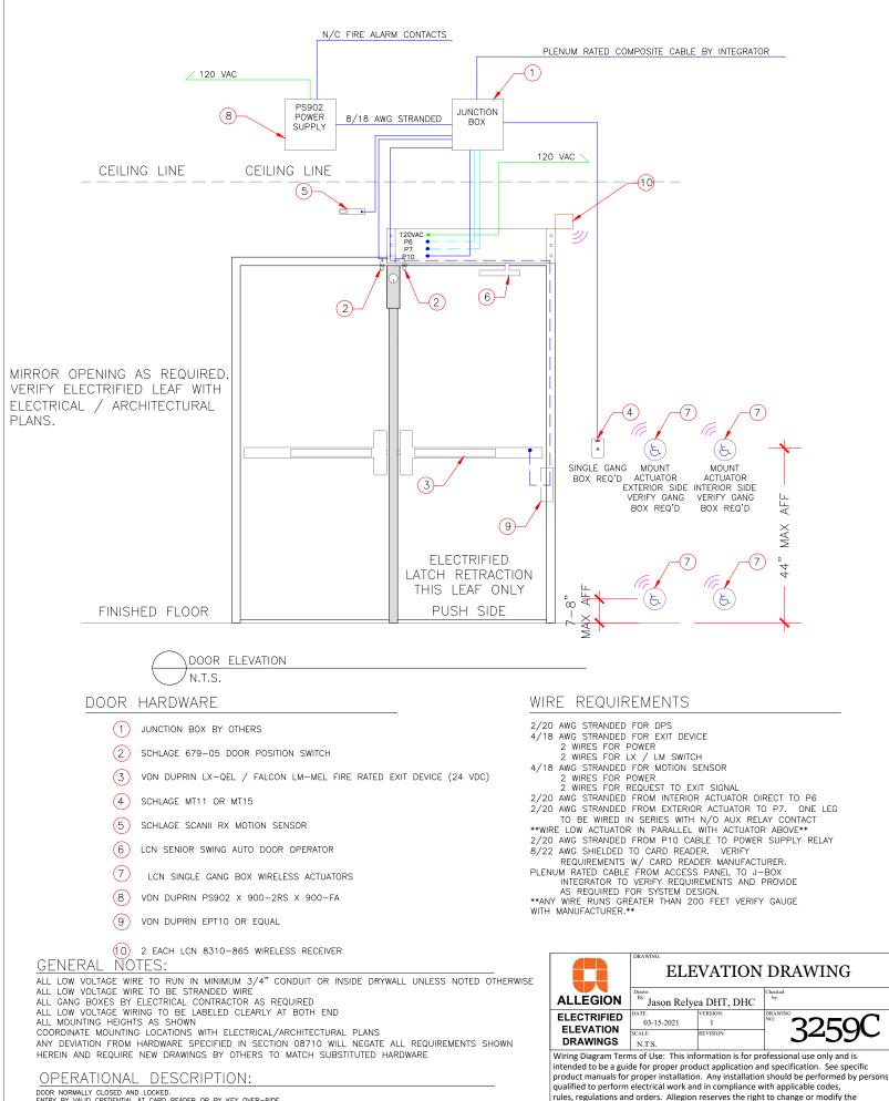
DOR NORMALLY CLOSED AND LOCKED. ENTRY BY VALID CREDENTIAL AT CARD READER OR BY KEY OVER-RIDE. RX MOTION SENSOR SHUNTS DOOR FORCED OPEN IN ACCESS CONTROL. SYSTEM. INTERIOR ACTUATOR TO START OPENING CYCLE (UNLESS ADD IS POWERED OFF) EXTERIOR ACTUATOR WIRED IN SERIES THROUGH LX SWITCH IN EXIT DEVICE SUCH THAT ON VALID CARD OR TIME ZONE CONTROL ACTUATOR CAN BE PRESSED TO START OPENING CYCLE KEY OVER-RIDE WILL CAUSE DOOR FORCED EVENT IN ACCESS CONTROL SYSTEM. FREE EGRESS AT ALL TIMES.
