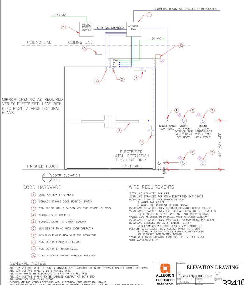
COORDINATE MOUNTING LOCATIONS WITH ELECTRICAL/ARCHITECTURAL PLANS ANY DEVIATION FROM HARDWARE SPECIFIED IN SECTION 08710 WILL NEGATE ALL REQUIREMENTS SHOWN HEREIN AND REQUIRE NEW DRAWINGS BY OTHERS TO MATCH SUBSTITUTED HARDWARE
