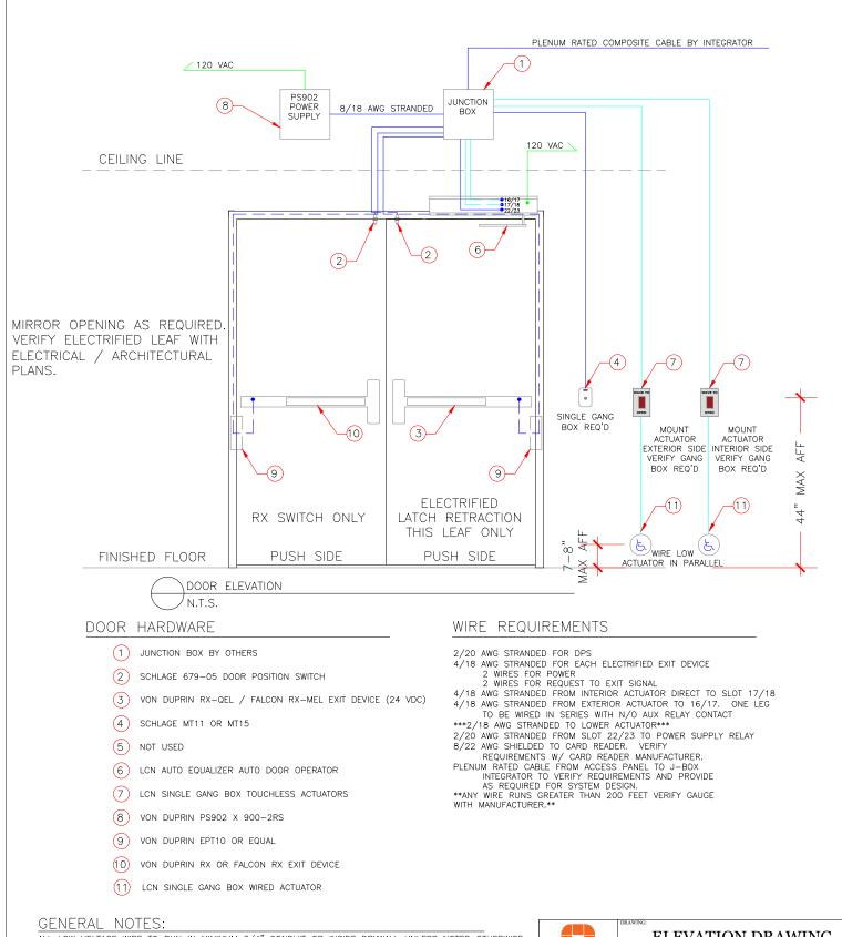
ALL LOW VOLTAGE WIRE TO RUN IN MINIMUM 3/4" CONDUIT OR INSIDE DRYWALL UNLESS NOTED OTHERWISE ALL LOW VOLTAGE WIRE TO BE STRANDED WIRE ALL GANG BOXES BY ELECTRICAL CONTRACTOR AS REQUIRED ALL LOW VOLTAGE WIRING TO BE LABELED CLEARLY AT BOTH END ALL MOUNTING HEIGHTS AS SHOWN COORDINATE MOUNTING LOCATIONS WITH ELECTRICAL/ARCHITECTURAL PLANS ANY DEVIATION FROM HARDWARE SPECIFIED IN SECTION 08710 WILL NEGATE ALL REQUIREMENTS SHOWN HEREIN AND REQUIRE NEW DRAWINGS BY OTHERS TO MATCH SUBSTITUTED HARDWARE
