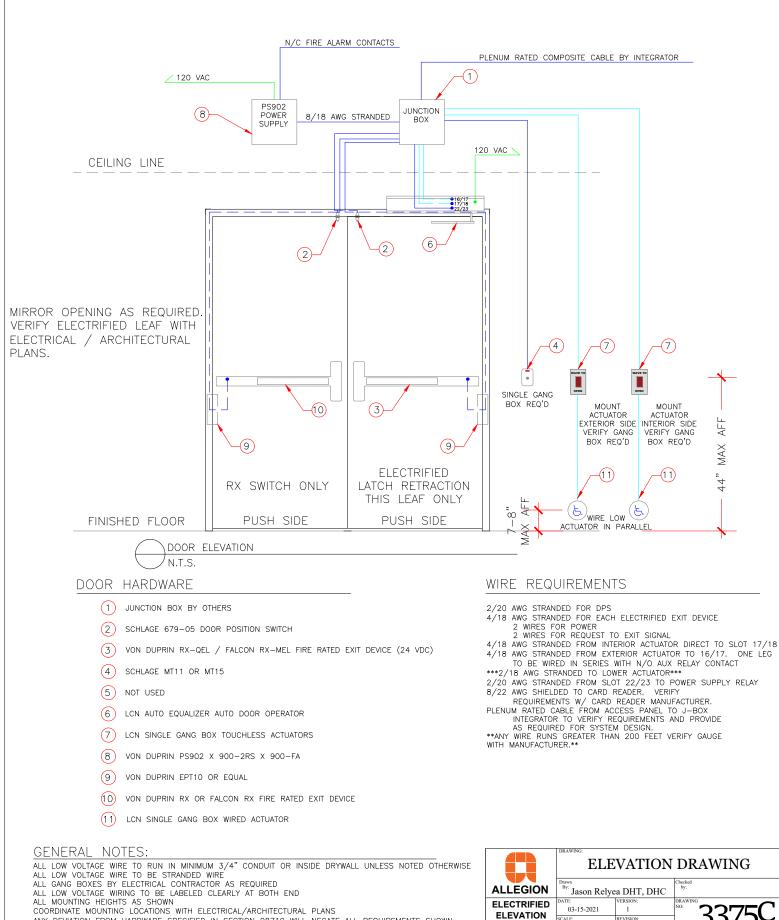
ANY DEVIATION FROM HARDWARE SPECIFIED IN SECTION 08710 WILL NEGATE ALL REQUIREMENTS SHOWN HEREIN AND REQUIRE NEW DRAWINGS BY OTHERS TO MATCH SUBSTITUTED HARDWARE
