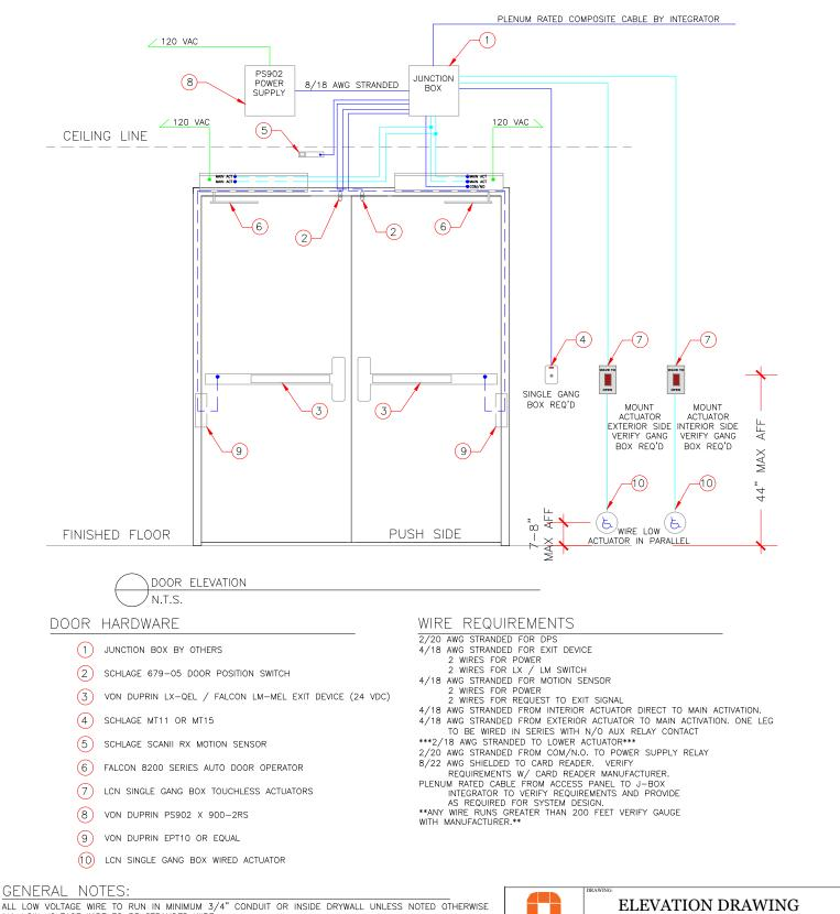
ALL LOW VOLTAGE WIRE TO BE STRANDED WIRE ALL LOW VOLTAGE WIRE TO BE STRANDED WIRE ALL LOW VOLTAGE WIRING TO BE LABELED CLEARLY AT BOTH END ALL MOUNTING HEIGHTS AS SHOWN COORDINATE MOUNTING LOCATIONS WITH ELECTRICAL/ARCHITECTURAL PLANS ANY DEVIATION FROM HARDWARE SPECIFIED IN SECTION 08710 WILL NEGATE ALL REQUIREMENTS SHOWN HEREIN AND REQUIRE NEW DRAWINGS BY OTHERS TO MATCH SUBSTITUTED HARDWARE
