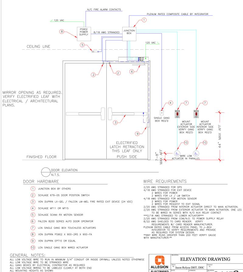
COORDINATE MOUNTING LOCATIONS WITH ELECTRICAL/ARCHITECTURAL PLANS ANY DEVIATION FROM HARDWARE SPECIFIED IN SECTION 08710 WILL NEGATE ALL REQUIREMENTS SHOWN HEREIN AND REQUIRE NEW DRAWINGS BY OTHERS TO MATCH SUBSTITUTED HARDWARE
