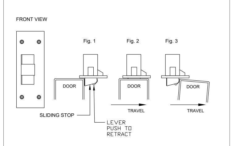
The #299 door stop is designed to convert pivot mounted single doors to double acting doors which allows the door to open in the opposite direction in the event the normal door opening is blocked by an obstruction.
