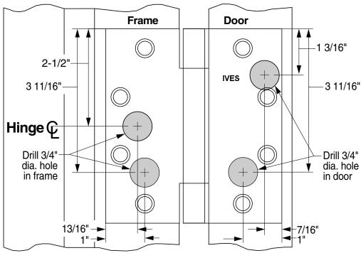
Notes: 1. Round Corners (RC) application will have 1/4" (6.35) and 5/8" (15.88) radius corners, but will conform to template as shown above the other radius corners.
