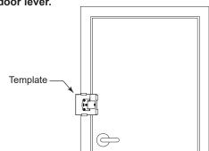
2. Make sure that the template is placed so that the edge of door guard will be offset 1/32" from edge of frame.
