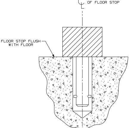
\*RECOMMENDED GROUT IS THOROGRIP AS MFD BY THORO SYSTEM PRODUCTS OR APPROVED EQUIVALENT
