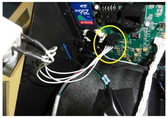
Remove the tamper switch connector from the main board. Do not pull by the wires but depress the tab to release the connector.
