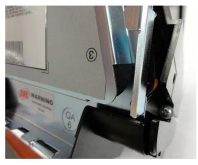
Pull the backup battery cable through the back plate as shown above.
