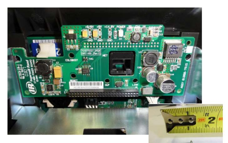
Secure the power board to the unit using the two screws shown in the image to the right.
