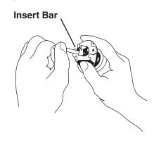
Install new spindle over bar, rotate slightly and push into place.
