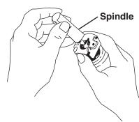
**8.** Position plunger button assembly onto bar and snap firmly into place. Snap On Button
