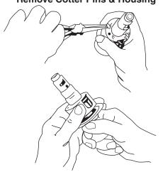
**5.** Depress slide, unhook old plunger by lifting, remove both plunger and spindle.
