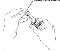
**9.** Replace housing and lock trim by reversing steps 1 thru 4.
