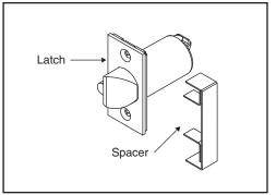
Position spacer on latch (as shown).
