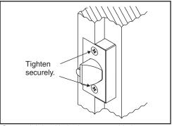
Secure tightly with the longest provided screws.
