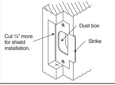
Insert dust box in hole. Place strike in position and secure to jamb with provided screws.
