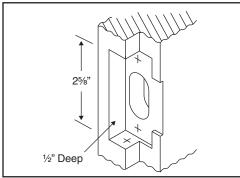
Cut away edge of door jamb for strike, dust box and shield.
