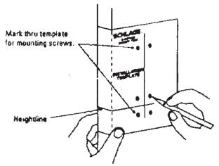
Place template on door at correct heightline and mark thru template for (6) mounting screws.
