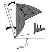
7. Hold the rear panel against the Handreader making sure that the rear panel has fit into the base properly. Rotate the Handreaders lock into the locked position.
