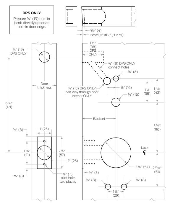
Dimensions shown in parentheses () are in millimeters.
