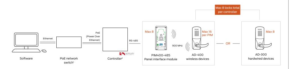
1 In order to have a UL Listed configuration a UL294 12VDC power supply must be used instead of PoE
