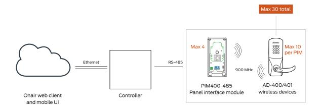
Wireless range up to 200' in typical building construction, up to 1000' line of sight
