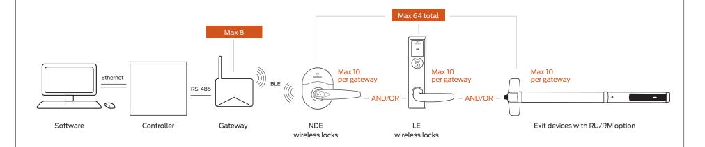
Gateway communication range up to 30' in typical building environments; a detailed site survey is recommended.
