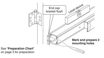
Install End Cap Bracket and End Cap
