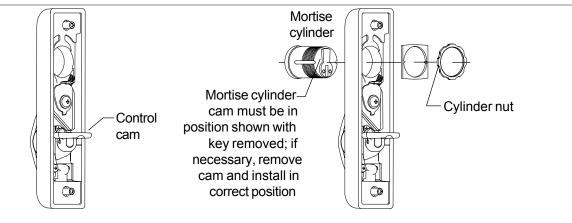
Figure 1. Control cam position.
