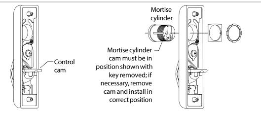
Figure 1. Control cam position.
