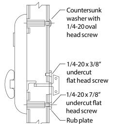
Figure 4. Control and rub plate application.
