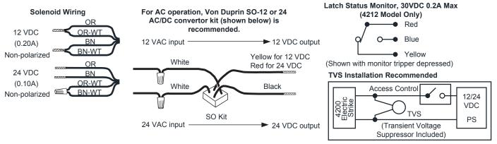
After installation, test strike by applying power to the solenoid. Fail Safe (FS) will lock the keeper. Fail Secure (FSE) will unlock the keeper.
