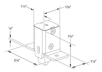
Soffit latch bolt assembly x2
