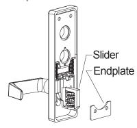
3 Push up on slider and pivot out to remove guide post assembly.
