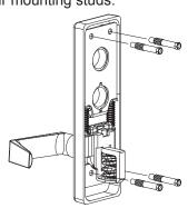
2 Remove endplate from under slider.
