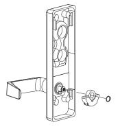
5 Use 3/32" hex wrench to loosen set screw. Remove shear pin.
