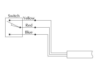
This switch is intended for signaling purposes only and is rated for a maximum 2 ampere resistive load at 24VDC/AC. Use with inductive or capacitive loads (magnetic locks or solenoid devices) derates the capacity of the switch. Consult the factory for assistance.
