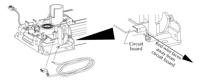
**B.** Place the cable in the channel on the underside of the device and run the pigtail end through the hole in the hinge side mounting plate.
