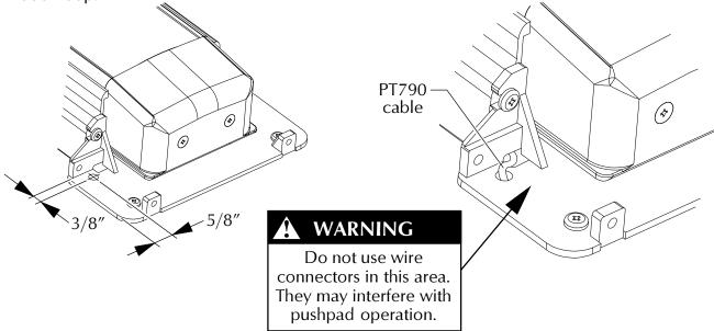
**C.** Connect PT790 cable wires to PT790 transformer leads using crimp connectors or wire nuts:
