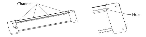
C. Continue with Step 6 of the GUARD-X installation instructions. Make sure that the PT790 cable stays in the channel when mounting device on door.
