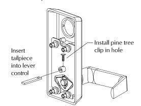
**4.** Prepare door for lever control installation.
