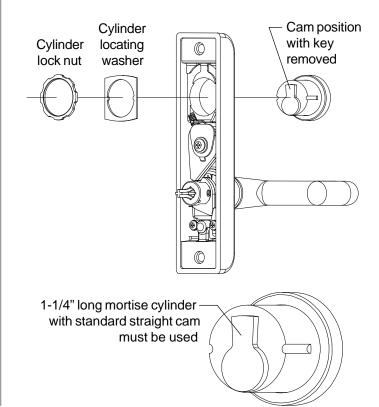
**4.** Prepare door for lever control installation.
