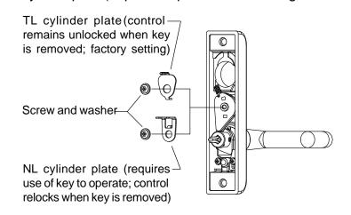
**3.** Install key cylinder as shown, then install the back plate that was removed in Step 1.
