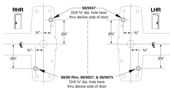
b. Prepare trim side of door using dimensions on front side of instruction sheet 921003/921006.
