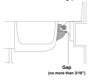
When properly adjusted, secure strike with additional screw.
