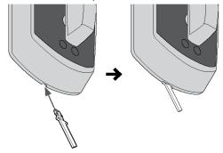
If the clip is not installing, flip it over and insert it at an angle the opposite direction (either right to left OR left to right).
