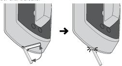
① You want the clip remaining in your deadbolt to be flush with the outside deadbolt assembly. If the breaking point extends below the outside deadbolt assembly, you may use an emery board or sand paper to file the clip to be flush with that assembly.
