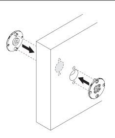
2 Install mounting posts and screws.
