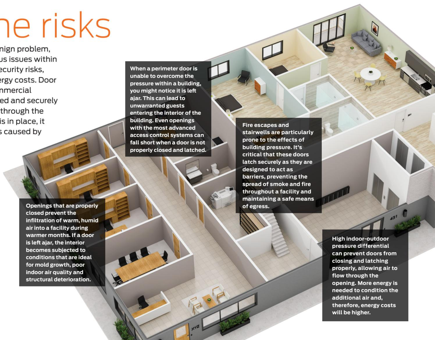
When a perimeter door is unable to overcome the pressure within a building, you might notice it is left ajar. This can lead to unwarranted guests entering the interior of the building. Even openings with the most advanced access control systems can fall short when a door is not properly closed and latched.
