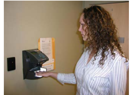
This reader, used at Community Hospice to collect time and attendance information, has an antimicrobial coating on its platen, where employees lay their hands.
