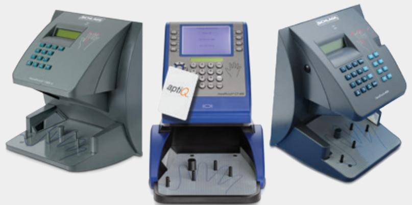
Hand geometry measures the size and shape of a user's hand to confirm identity. Over 90 distinct measurements are made each time to verify a user. These include length, width, thickness and surface area. It does not read fingerprints or palm prints.
