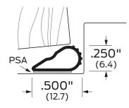
Notes: Intumescent rubber for fire and smoke protection. PSA standard. 45-minute fire rating.
