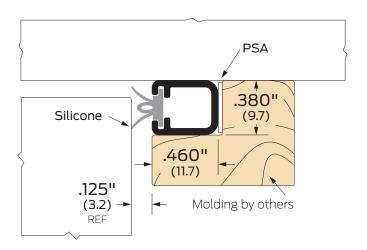
**Notes:**For applications with very small clearances between door and frame. Supplied standard with PSA.
