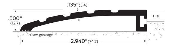
Notes: Also suitable for use as carpet divider threshold. ADA compliant when installed flush with the flooring
