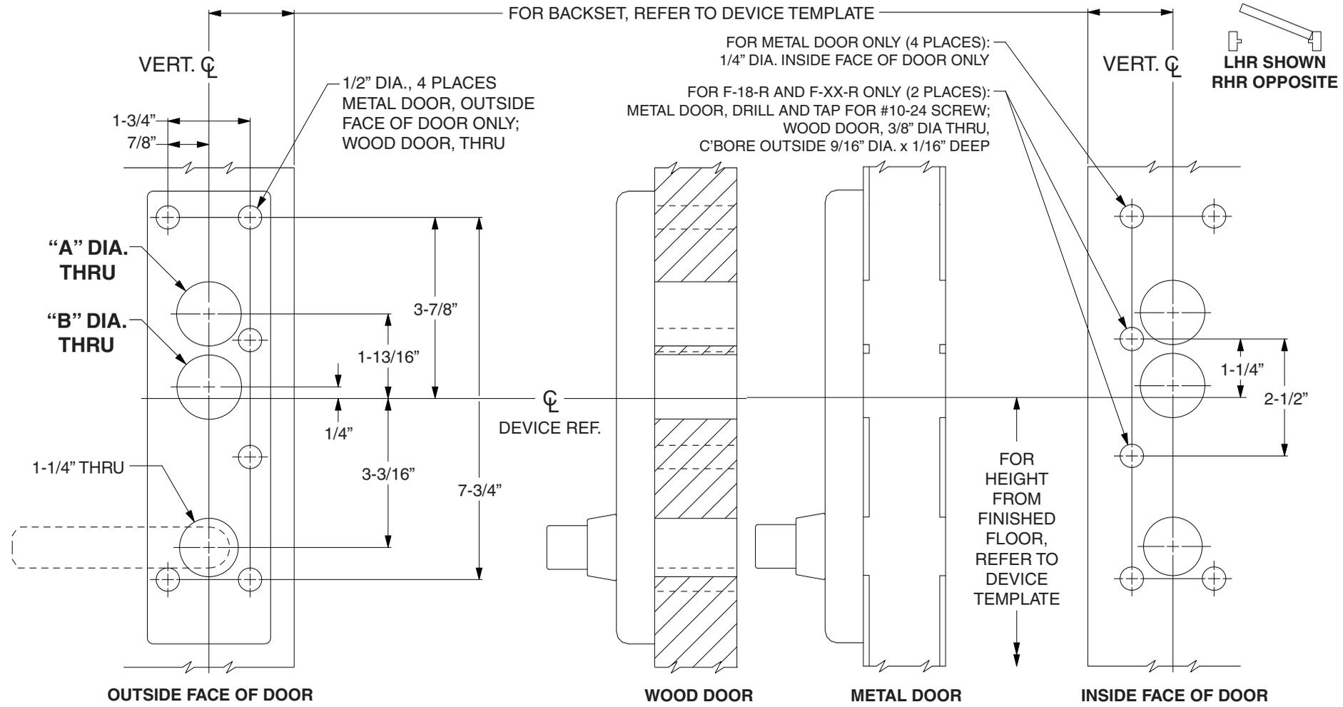
1. PREPARE INSIDE FACE OF DOOR FOR DEVICE. SEE DEVICE DIRECTIONS FOR LOCATIONS OF VERT. AND DEVICE REF. CENTER LINES.
