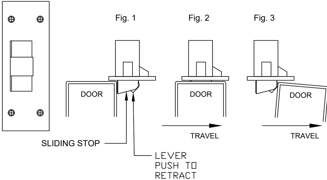
The #299 door stop is designed to convert pivot mounted single doors to double acting doors which allows the door to open in the opposite direction in the event the normal door opening is blocked by an obstruction.
